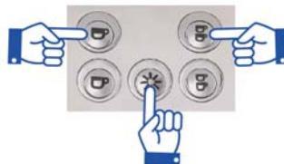
Keep it pressed and move the main switch of the machine in position 1 or 2, is indistinct. Hold it for several seconds until visualizar onscreen display **RESET COMPLETE** message.
