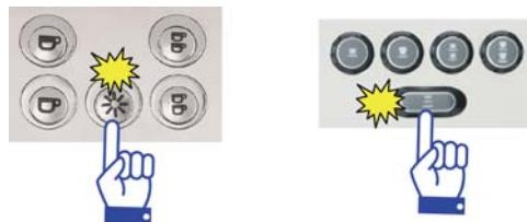
At this point programming can be started for the four coffee selections. When the desired quantity of coffee is obtained, press the selection once again and the dosing will stop. The same operation will have to be followed for all buttons.
